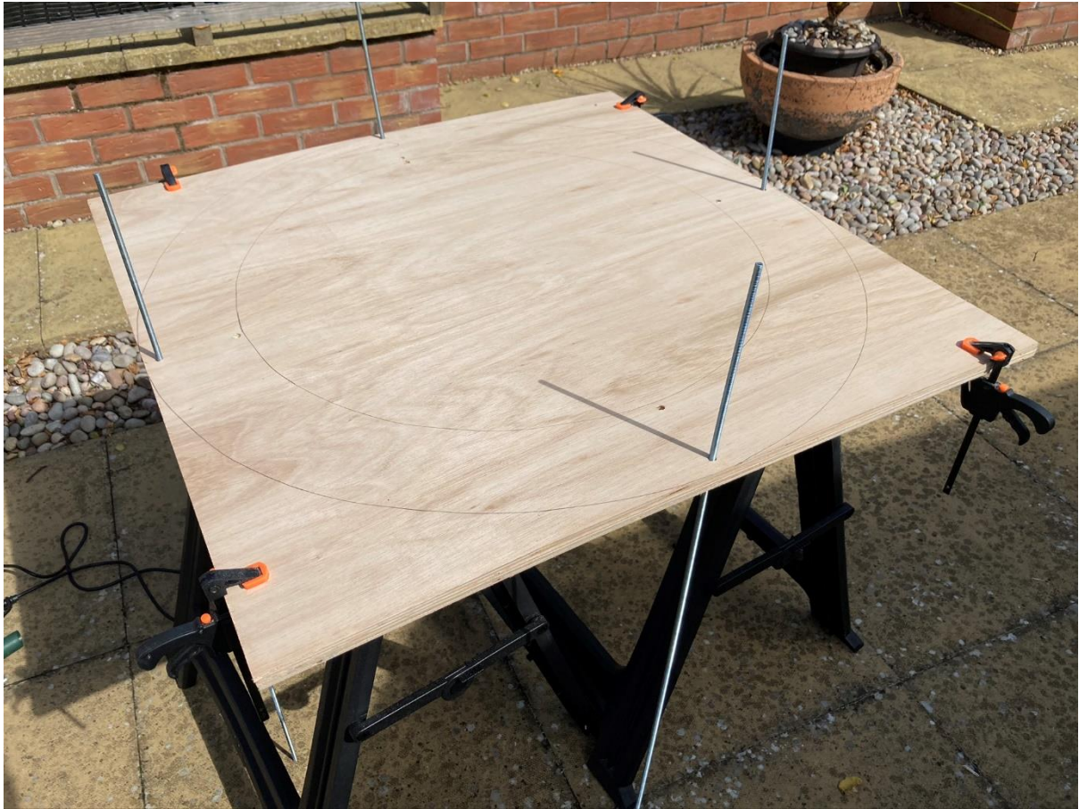
Figure 7 - Aligning the Cutting Set Before Sawing
