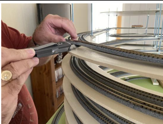
Figure 39 - Re-Lifting the Glued Track
