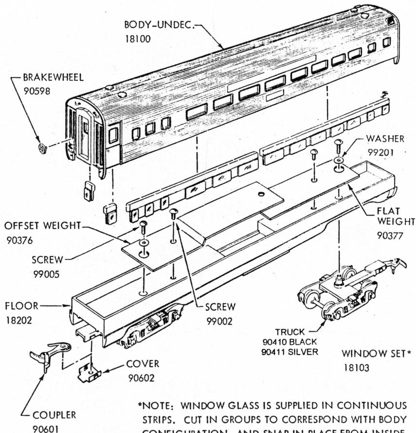
\*NOTE: WINDOW GLASS IS SUPPLIED IN CONTINUOUS STRIPS. CUT IN GROUPS TO CORRESPOND WITH BODY CONFIGURATION, AND SNAP IN PLACE FROM INSIDE BODY BY ENTERING BOTTOM EDGE OF GLASS OVER LIP IN WINDOW SILL. CEMENTING IS NOT REQUIRED.
